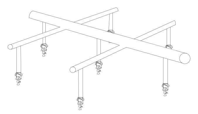
Figure 8. Example Spray Header Liquid Distributor
