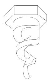
Figure 9. Example Full Cone Spray Nozzle with Maximum Free Passage
