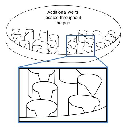
Figure 6. Example Weir Riser Pan Distributor
