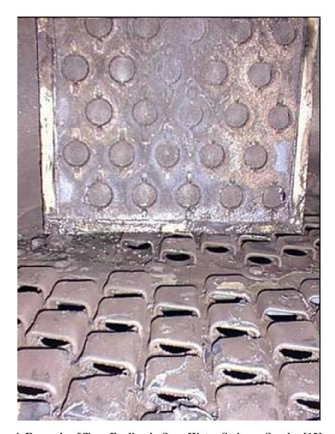
Figure 4. Example of Tray Fouling in Sour Water Stripper Service [12].
