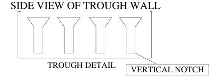
Figure 7. Sketch of Trough Style Distributor
