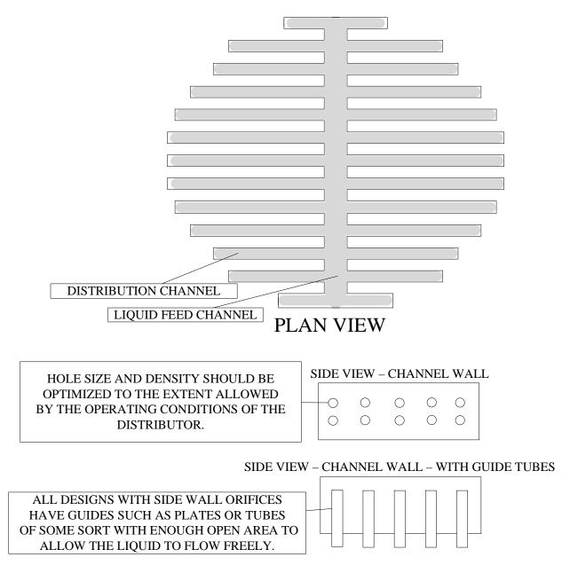
Figure 5. Example Channel-Type Distributor
