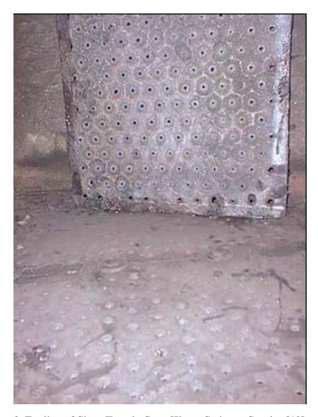
Figure 3. Fouling of Sieve Tray in Sour Water Stripper Service [12].
