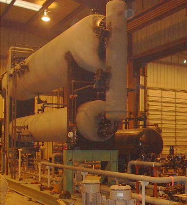
Figure 2 – Process Modules for Glycerol Dehydration in Fabrication
