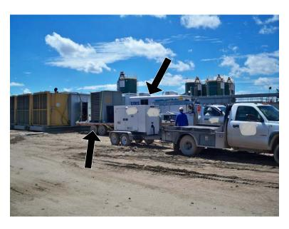
Figure 10 Load Bank (left) and URS Testing Trailer (back)
