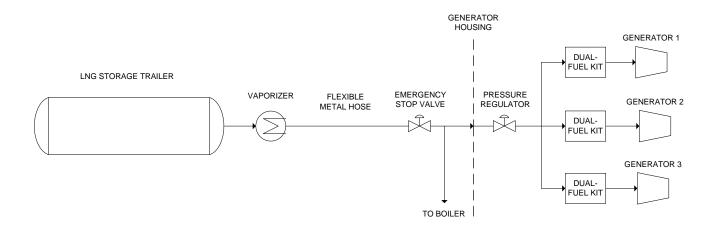
Figure 1 Overview Schematic of LNG System
