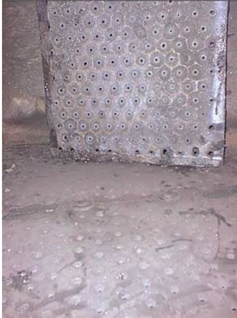
Figure 3. Fouling of Sieve Tray in Sour Water Stripper Service [13].
