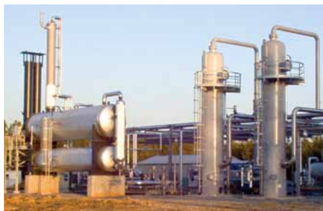
FIG. 2A Example sources of high-purity CO 2 and low H 2 S streams—CO 2 dehydration unit.
